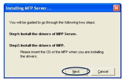
6. When you are installing the MFP Server Drivers, the following message will be displayed to notify you. When the MFP Server drivers are all installed, the message will be disappeared automatically.
